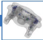
Automatic NDT pore volume analysis.
