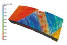
Metrology: Coordinate Measurement with integrated CAD Nominal/Actual Comparison
