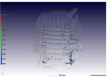
Figure 1: 3D analysis of radio controlled airplane engine casing with lots of porosity, only defects >1mm are highlighted here. More images and videos on the website (link to the left)
