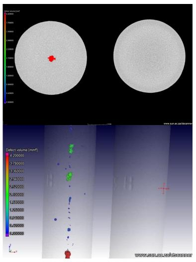
Figure 3: Porosity analysis before and after HIP treatment (same sample) – max pore diameter was 3 mm before HIP.
