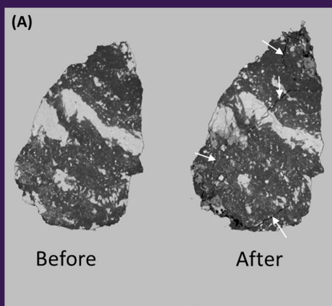
FIG 3: X-ray CT scan of particle before and after microwave treatment
