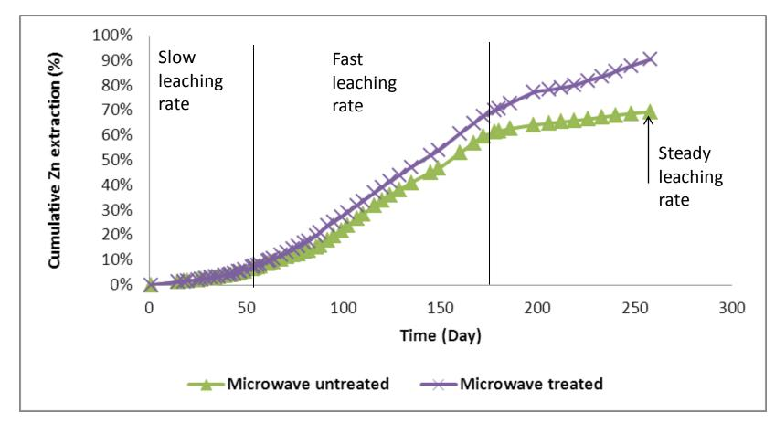
Cumulative Zn recovery of HPGR (-5+4.75)mm crushed particles
