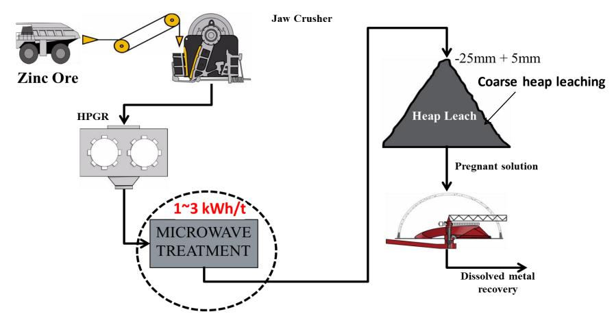
• Develop optimal energy efficient flow sheet for exploiting microwave induced grain boundary fractures
