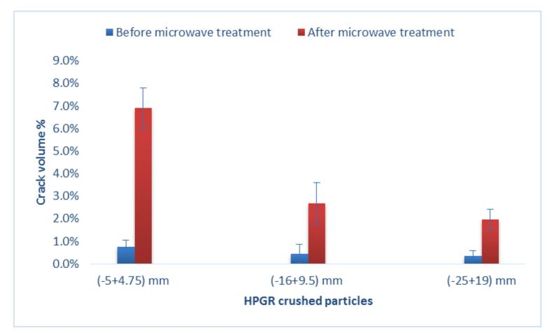
Mean crack volume values and standard deviation for HPGR crushed particles before and after microwave treatment
