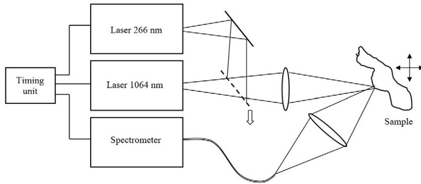
Fig. 1. LIBS experimental set-up.
