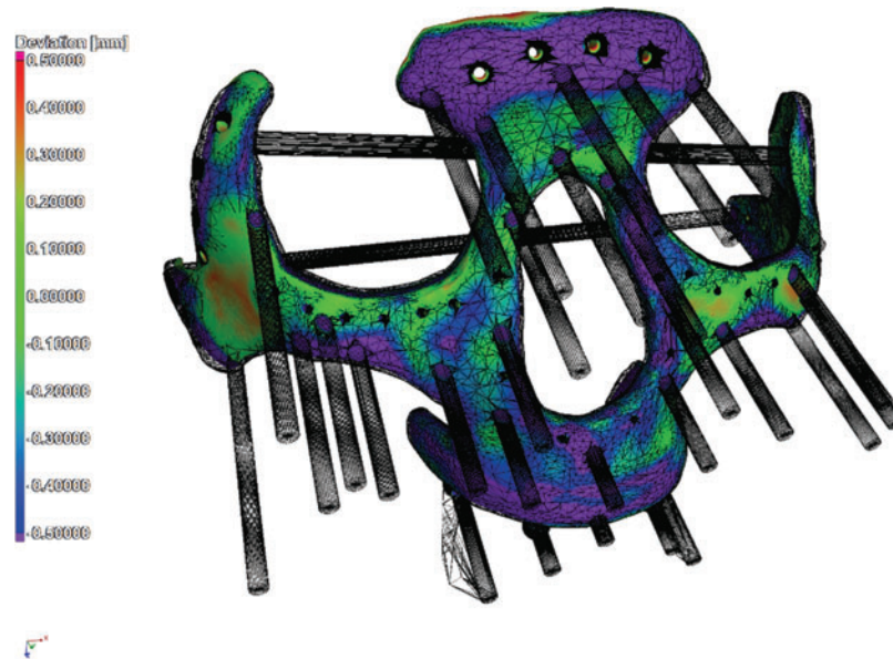
FIG. 6. CAD variance analysis of facial implant built by LPBF—CAD file mesh includes supports. Blue areas are smaller than design, red are larger. CAD, computer-aided design. Color images available online at www.liebertpub.com/3dp
