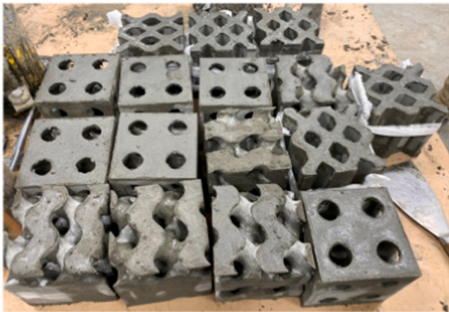
Fig. 8. Cast concrete lattice structures, produced by casting in plastic 3D-printed molds [64].
