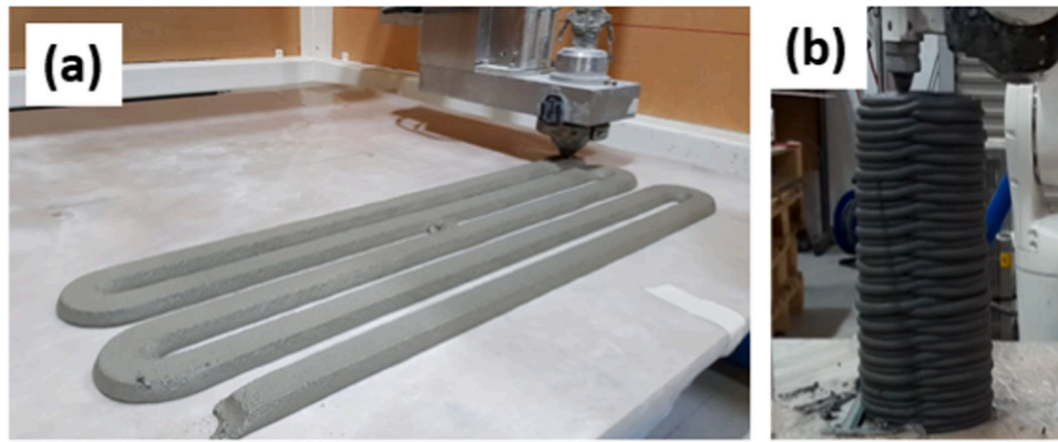
Fig. 11. (a) extrudability and (b) buildability in 3D concrete printing process [116].
