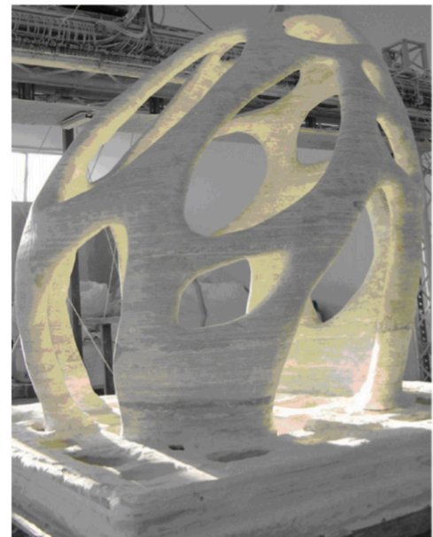
Fig. 15. Architectural piece by D-Shape process [132,133].
