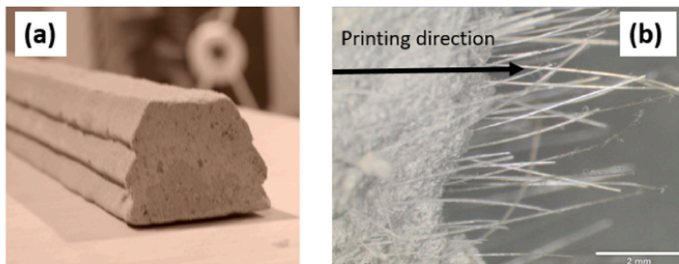
Fig. 12. Fracture image of (a) 3D-printed sample and (b) aligned fiber in the printing direction.
