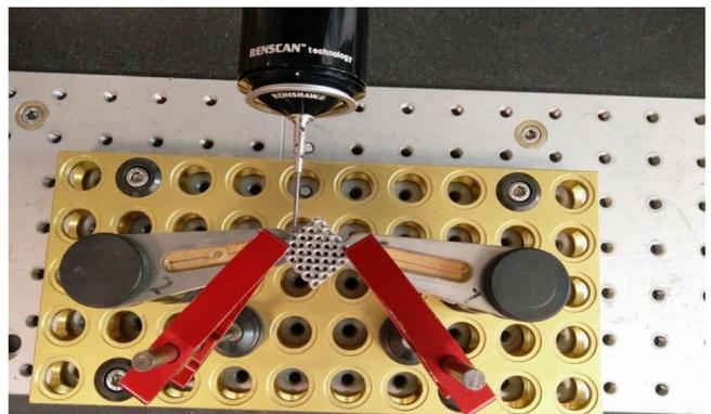
**FIGURE 5** Clamping configuration of lattice gyroid sample in the coordinate measurement machine (CMM) working plane
