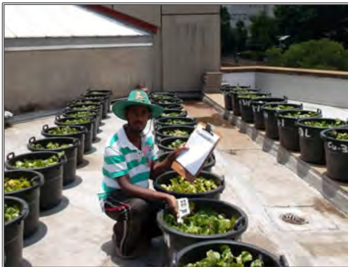
Figure 15: Dr Solomon Newete from the University of the Witwatersrand measuring the removal of metal salts from water by the invasive weed, water hyacinth ( Eichhornia crassipes ) (Image: Solomon Newete)
