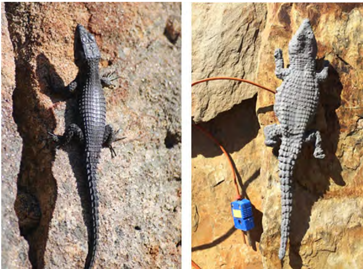
Figure 13. To measure the habitat temperatures available to Cordylus oelofseni (left), the study's authors used 'operative temperature models' (right). These models were hollow copper replicas of the lizards, with a temperature sensor inside that was connected to a central data logger. By mimicking the thermal properties of live organisms in the absence of physiological function, these models can accurately predict the temperature that a live organism would experience in the same location. (Photos by Raquel A. Garcia)
