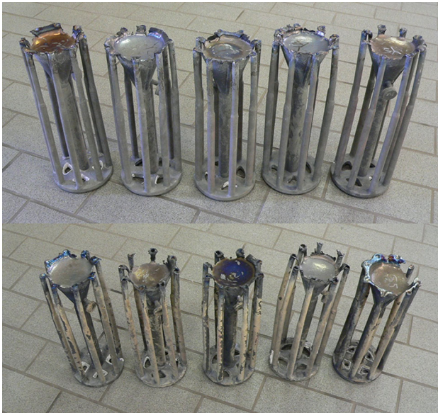
Fig. 2 Sample rods after casting with mold removed
