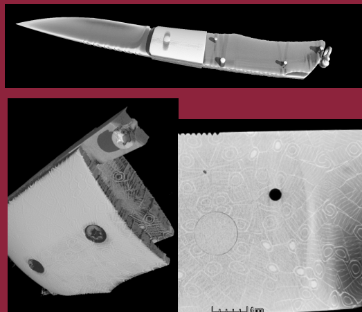
Damascus steel knife – CT scans show internal patterned structure of the steel
