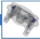
Automatic NDT pore volume analysis.
