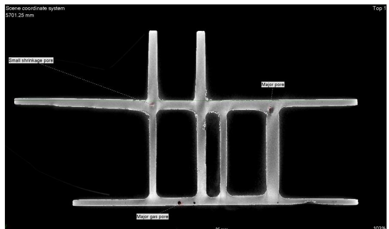
Figure 1: Titanium aerospace investment casting analysis
