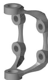
Figure 8: smoothed TO part generated utilizing PolyNURBS
