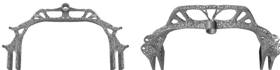
Figure 21: Smoothed Topology Optimized and Latticed steering arch, including solid 'shell' sections for support material connection (l) for upright orientation, and (b) for face-down
