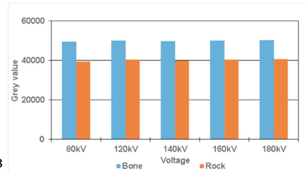
**Figure 4.** Effect of voltage change on scan quality evaluated by (A) visual impression in CT slice images and (B) grey values of representative regions of fossil bone and rock.
