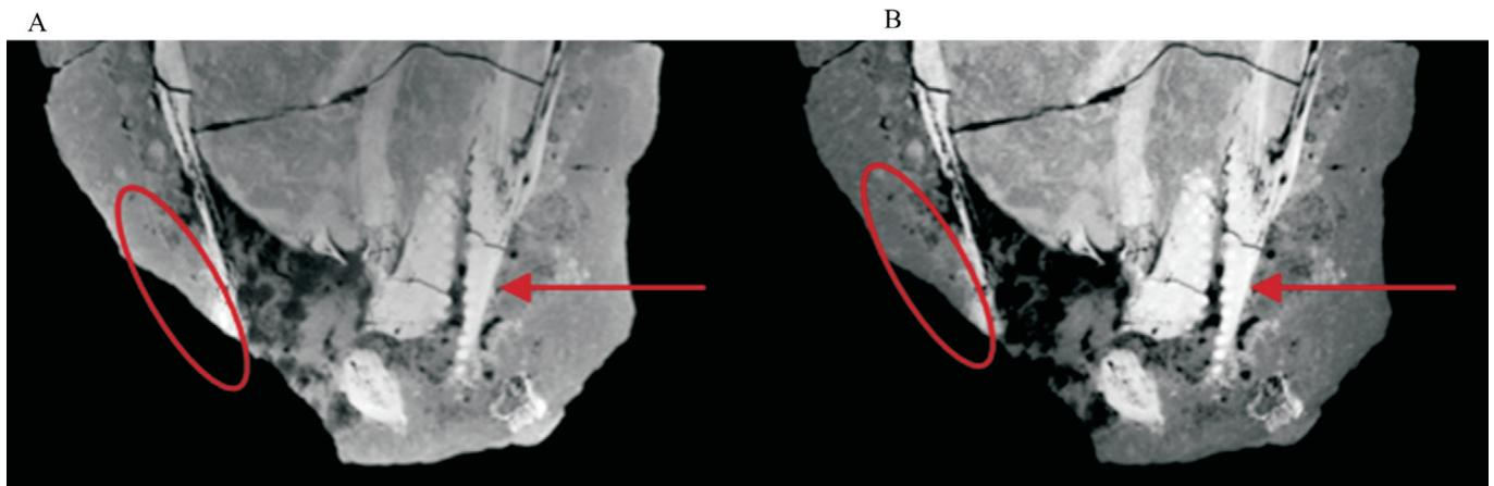
**Figure 11.** 2D slice images showing the results of beam hardening on a sample (A) vs a beam hardening corrected 2D slice image of the same data set (B). The cupping effect on the sample is shown by the red circle on the left slice image and the corrected cupping by the red circle on the right. The arrows point on the dark interior of the sample as result of beam hardening (A) and corrected beam hardening interior of the sample (B).
