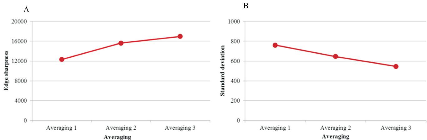
**Figure 14.** The effect of varying averaging on the image edge sharpness measured as the gradient of the slope between two materials, using the minimum and maximum values of the two (A) and background noise measured as the standard deviation of the mean grey values taken from the volume of the ROI (B).
