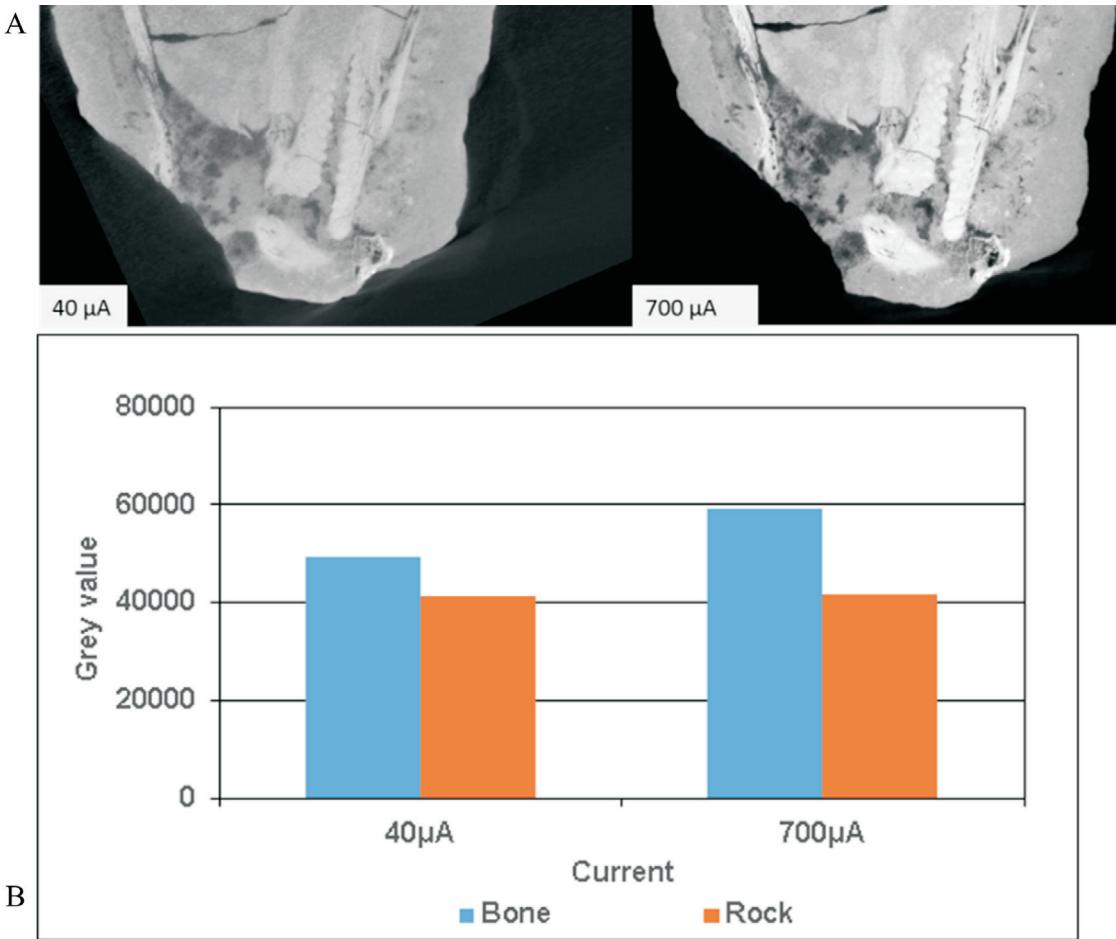
**Figure 7.** Increased current shows improved quality as evaluated by (A) 2D slice images and (B) grey values of representative regions of fossil bone and rock.
