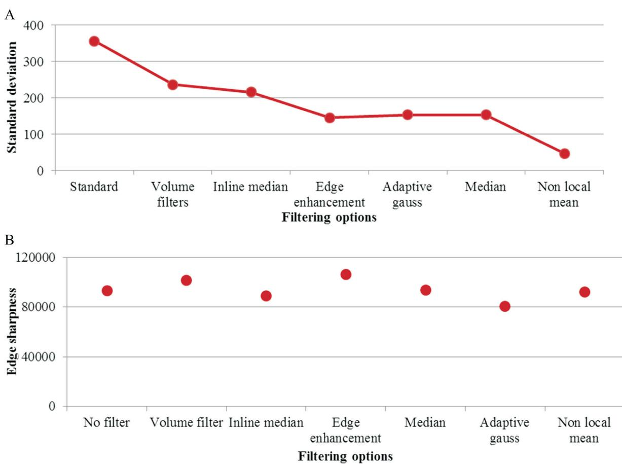
**Figure 15.** The effect of varying filtering options on the image edge sharpness measured as the gradient of the slope between two materials, using the minimum and maximum values of the two (A) and background noise measured as the standard deviation of the mean grey values taken from the volume of the ROI (B).
