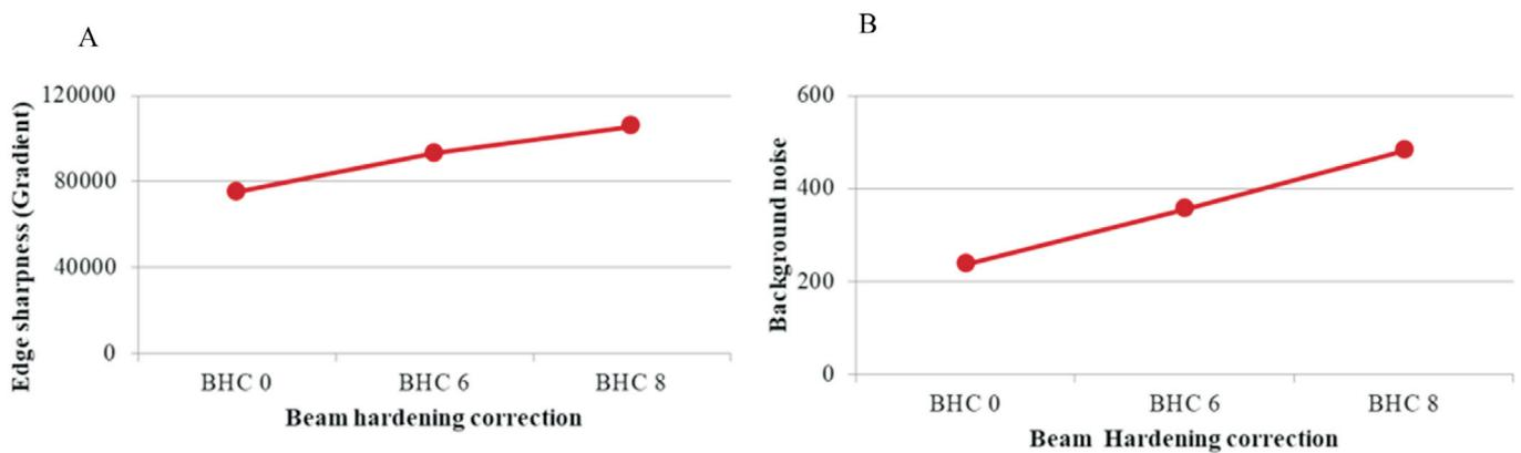
**Figure 12.** The effect of varying beam hardening correction on the image edge sharpness measured as the gradient of the slope between two materials, using the minimum and maximum values of the two (A) and background noise measured as the standard deviation of the mean grey values taken from the volume of the ROI (B).
