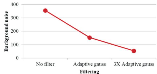
**Figure 16.** The effect of on increasing filtering on the image edge sharpness measured as the gradient of the slope between two materials, using the minimum and maximum values of the two (A) and background noise measured as the standard deviation of the mean grey values taken from the volume of the ROI (B). (A, Left) Unfiltered scan (B, middle) is the adaptive gauss and (C) is the 3X adaptive gauss filtered slice image.
