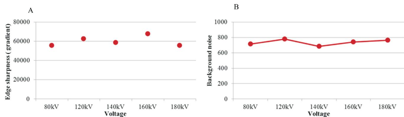
**Figure 5.** The effect of varying voltage on the image edge sharpness measured as the gradient of the slope between two materials (A) and background noise measured as the standard deviation of the mean grey values taken from the volume of the ROI (B).
