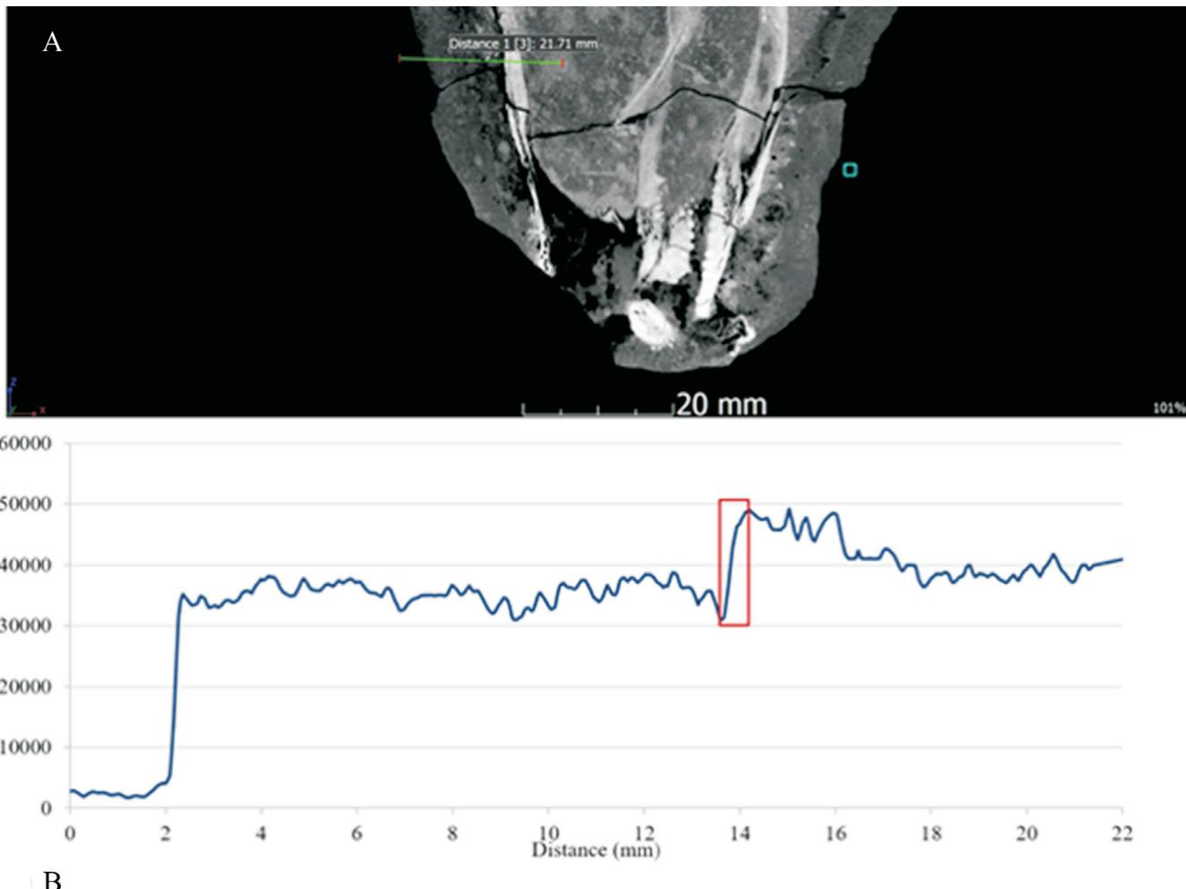
**Figure 3.** 2D slice image of SAM PK K10180 showing the region of interest for background noise measurement (blue block) (A) and the line profile taken across the fossil bone – rock interface for edge sharpness measurement. The red box on the line profile indicates where the edge sharpness was calculated and the green line in the CT image shows where the line profile was taken (B).
