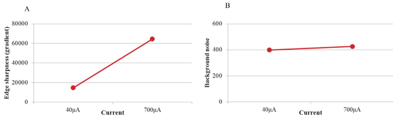
**Figure 8.** The effect of varying current on the image edge sharpness (A) and background noise (B).
