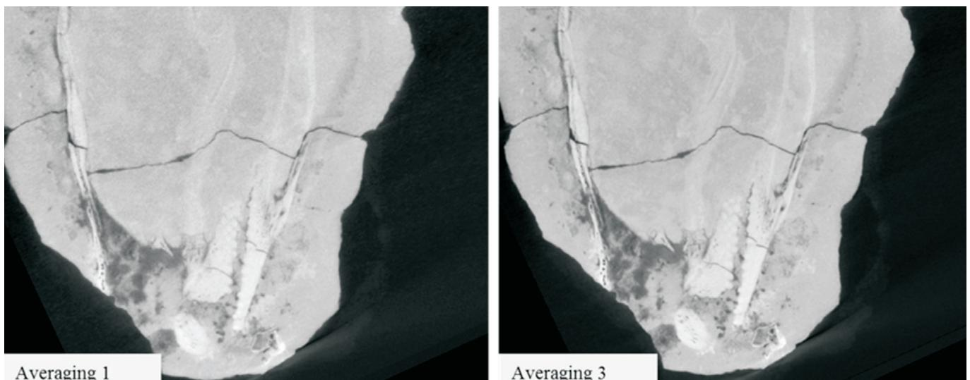
**Figure 13.** 2D slice images showing the quality change of varying image averaging.
