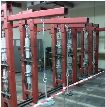
Figure 10. a) The tensile creep test setup.
