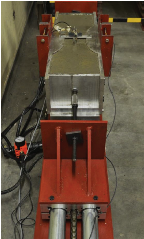
Figure 7. a) The tensile test setup for fresh concrete.
